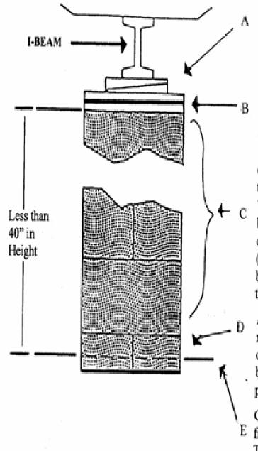
Pressure treated shims shall be fitted and driven tightly between the wood plate and main frame. Shims shall not occupy more than one (1) inch of vertical space.
